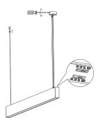
3. Connect the wires, then tighten the screws; As shown in the picture above:
